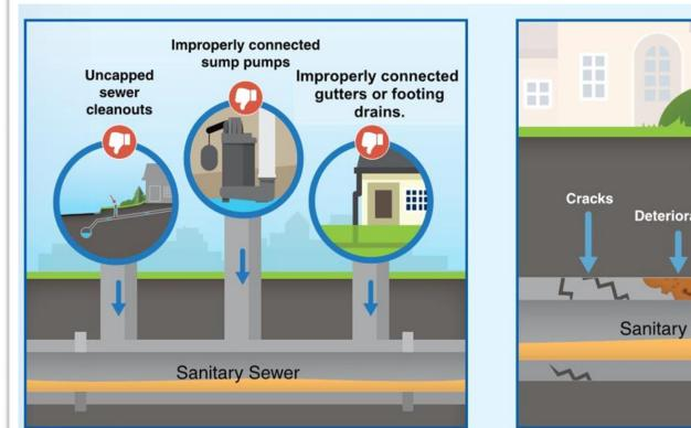
**Inflow** is clear water that quickly enters the wastewater system after rainfall events from sources such as sewer cleanouts, sump pumps, gutters, building foundation drains, and broken maintenance hole covers.
