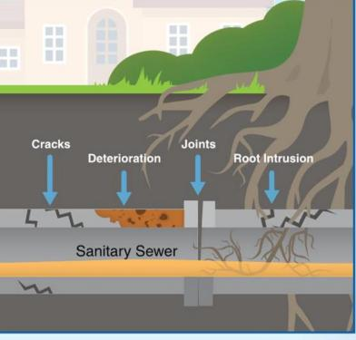
**Infiltration** is clear water that gradually enters the wastewater system below ground through cracks and openings in sewer service lines and joints, and public sewer mains and deteriorated maintenance holes.
